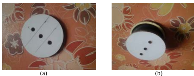
Fig. 2. Wheel construction from Ebonite sheet (a) Single wheel (b) Complete wheel.
