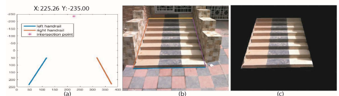
Fig. 9. Experimental example of stairways region detection: a) measuring VP, b) detected ROI in original image, and c) final detected stairways region.
