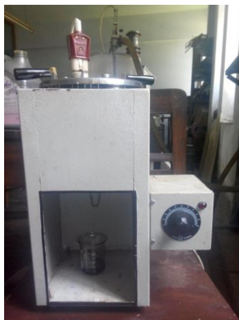
Fig. 2. Saybolt viscometer for viscosity measurement
