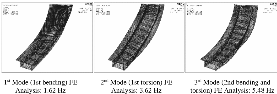
Figure 2.3: Different mode shapes and natural vibration frequencies
