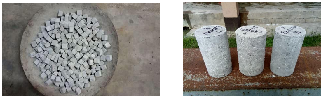
Figure 2: Artificial Aggregate and Concrete Incorporated with Artificial Aggregate
