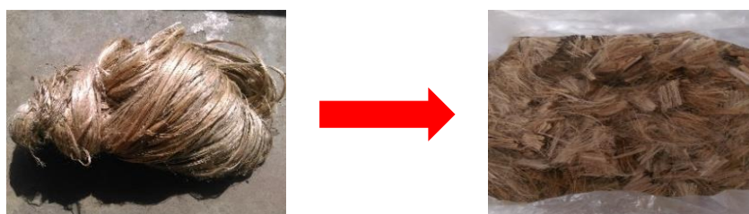
(a) Jute fibres cut into small pieces (Approx.12 mm in length)
