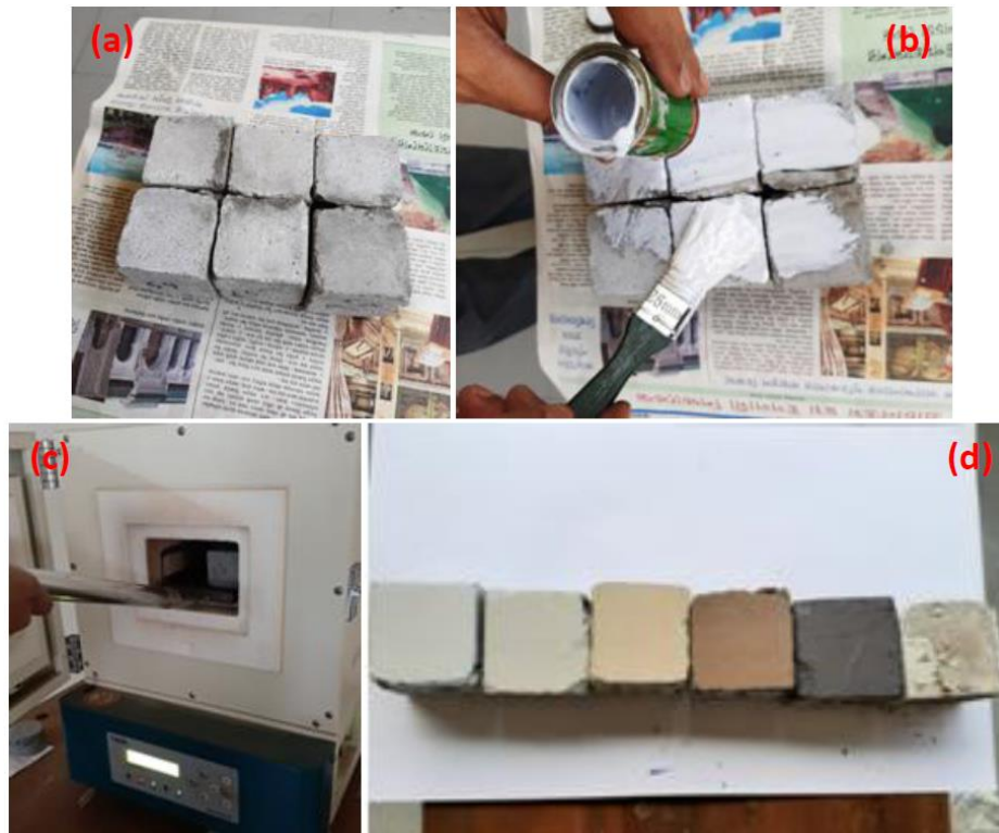
Figure 1: Experimental setup, a) plaster samples, b) enamel painting, c) electrical furnace and d) heated samples
