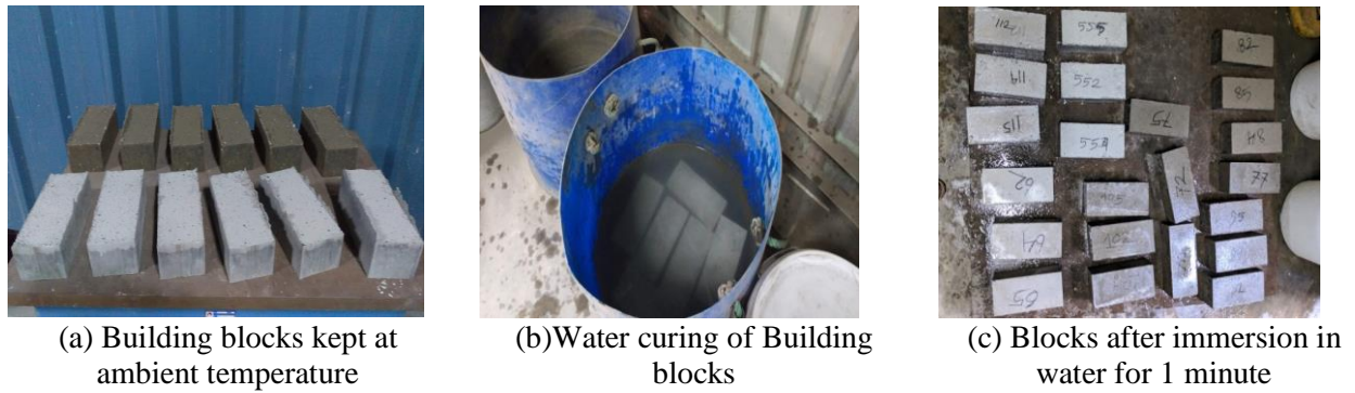
Figure 5: Curing process of building blocks
