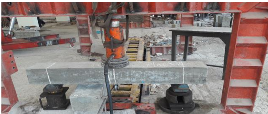
Figure 4: Typical test setup for flexural strength of reinforced concrete beam
