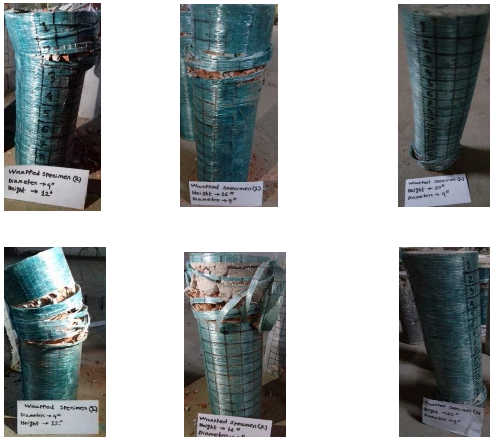
Figure 9: Failure pattern of wrapped cylindrical specimens.
