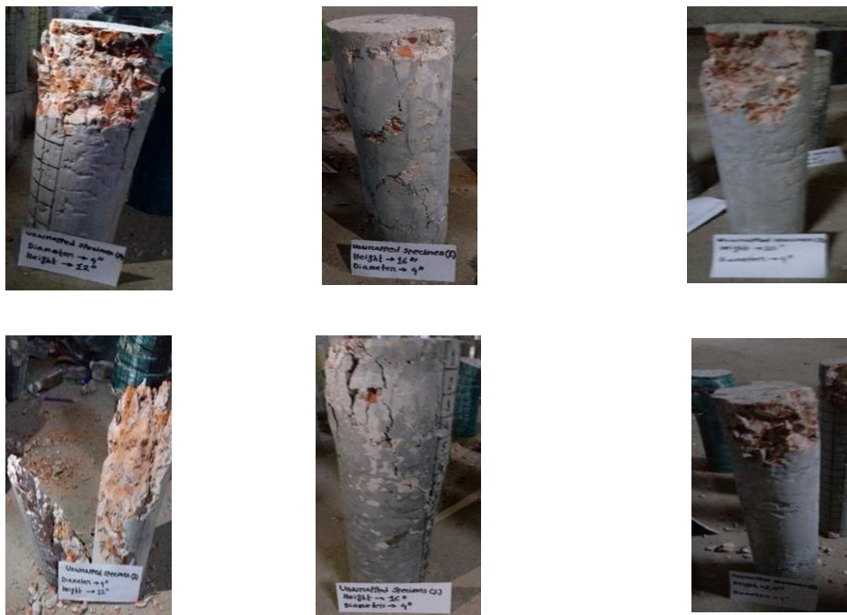
Figure 8: Failure pattern of unwrapped cylindrical specimens.
