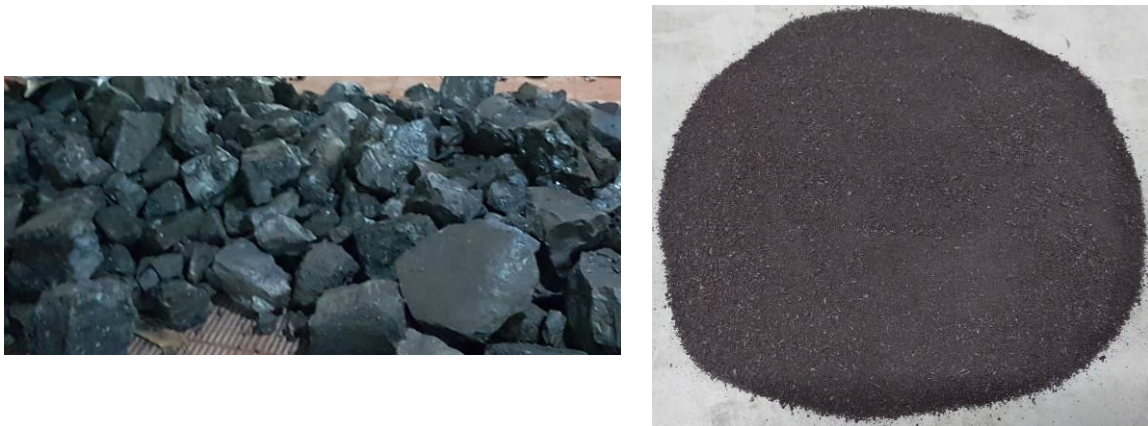
Figure 1: Steel slag chunks (left) and steel slag fine aggregate (right), respectively.
