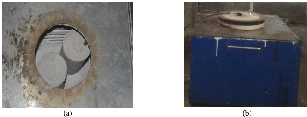
Figure 2: (a) Placement of the specimens in the furnace, (b) Furnace during heating process
