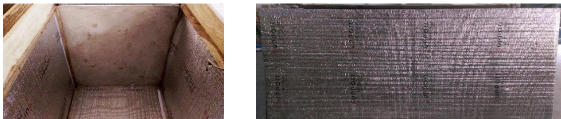
Figure 6: Insulation of box with PE foam
