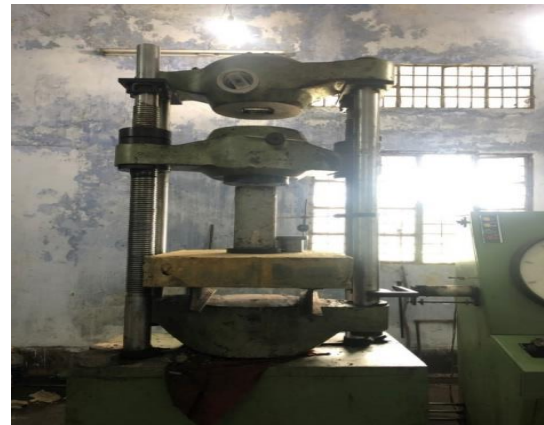
Fig. 9: Details view of experimental test setup in universal testing machine
