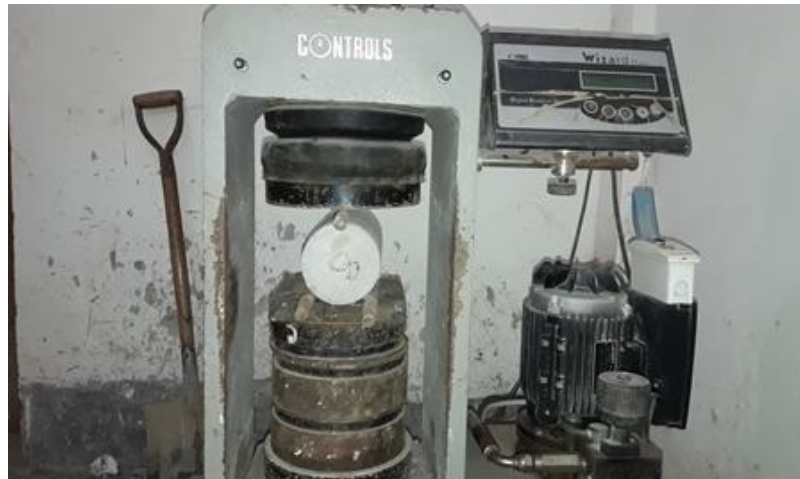
Figure 6: Typical setup for splitting tensile strength determination
