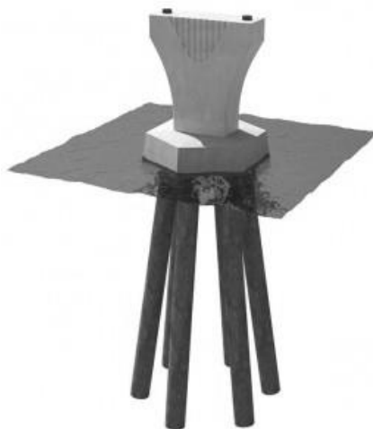
Figure 4: View of pile Layout (UNB)
