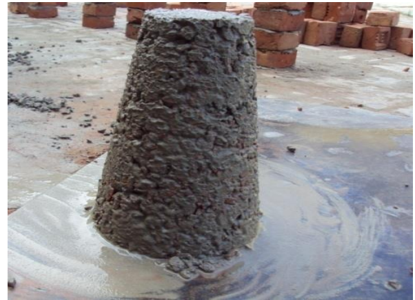
Fig. 4: Slum value test of M20 grade concrete
