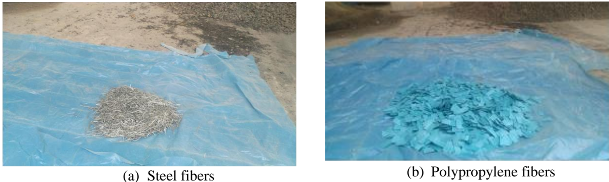
Figure 2: Appearances of polypropylene fibers and steel fibers
