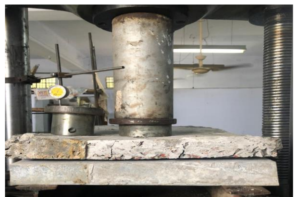
Fig.13: Plate end interfacial debonding
