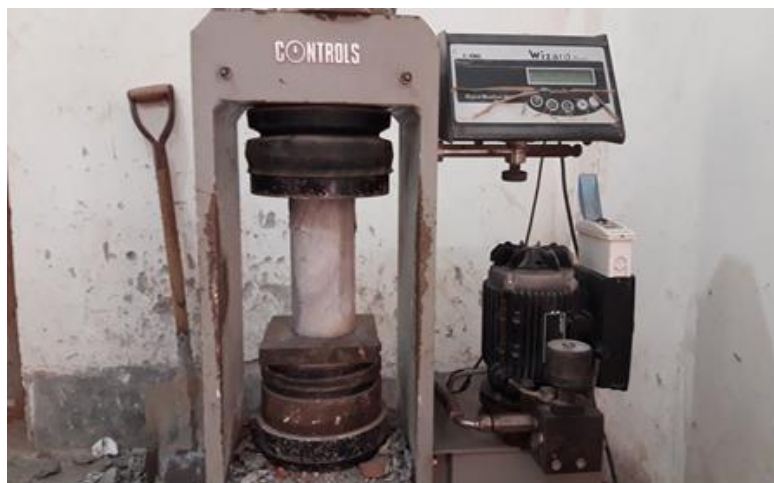
Figure 5: Typical test set-up for determination of crushing strength of concrete
