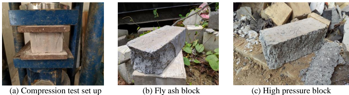
Figure 6: Compressive strength test and failure planes of building blocks
