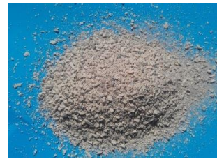
Figure 4: Appearance of Fine Aggregate from Waste Tiles
