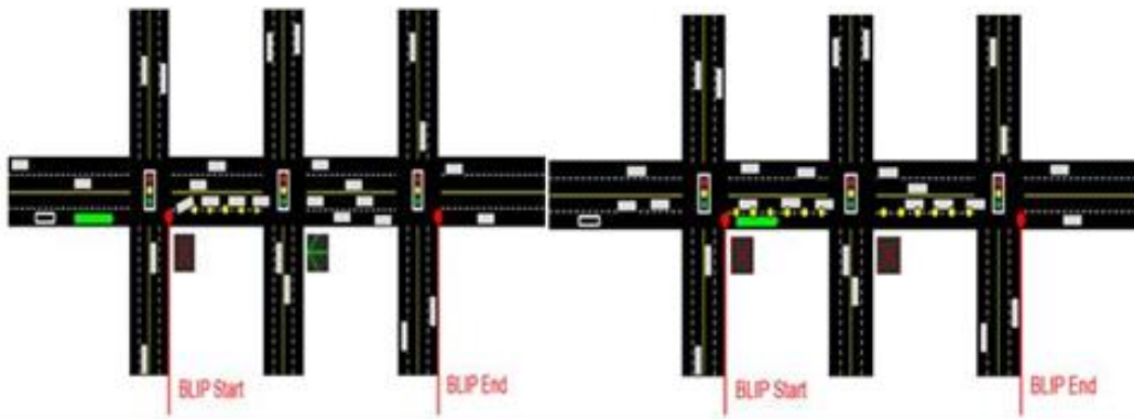
Figure 6: (a) Step 3: General traffic leaving BLIP lane; (b) Step 4: Bus enters cleared BLIP lane (Eichler and Daganzo, 2006).
