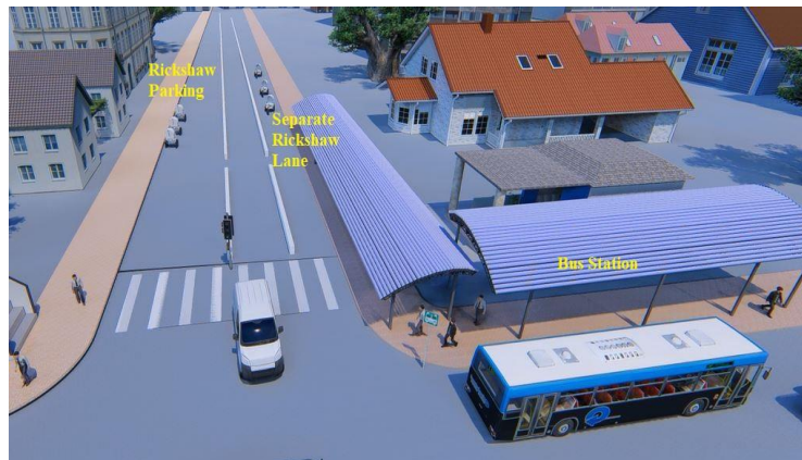
Figure-8: Demonstration of separate rickshaw lane, rickshaw parking, bus station and modal integration arrangement
