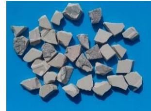
Figure 2: Appearance of Waste Tiles Aggregate
