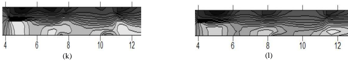
Figure 7: Velocity field of groin field measured by Surfer for series-1, case-1. (a)L/l=1; (b)L/l=2; (c)L/l=3; (d)L/l=4; (e)L/l=5; (f)L/l=6; (g)L/l=7; (h)L/l=8; (i)L/l=9; (j)L/l=10; (k)L/l=11; (l)L/l=12.
