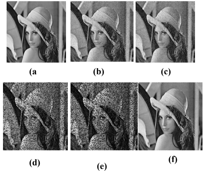
Fig. 4: Restoration of Lena image. (a) Original image, (b) Corrupted image with Salt & pepper noise (16.1023 dB), (c) Image recovered by AMF technique (24.4312 dB), (d) Image recovered by GMF technique (11.1253 dB), (e) Image recovered by HMF Technique (10.9820 dB), (f) Image recovered by TSAMFT (t = 60) (31.0934).
