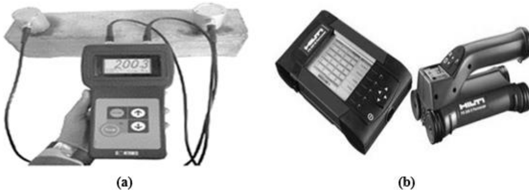
Fig. 2: (a) Ultrasonic Concrete Testing Instruments (b) Hilti PS 200 Monitor and Scanner Device.
