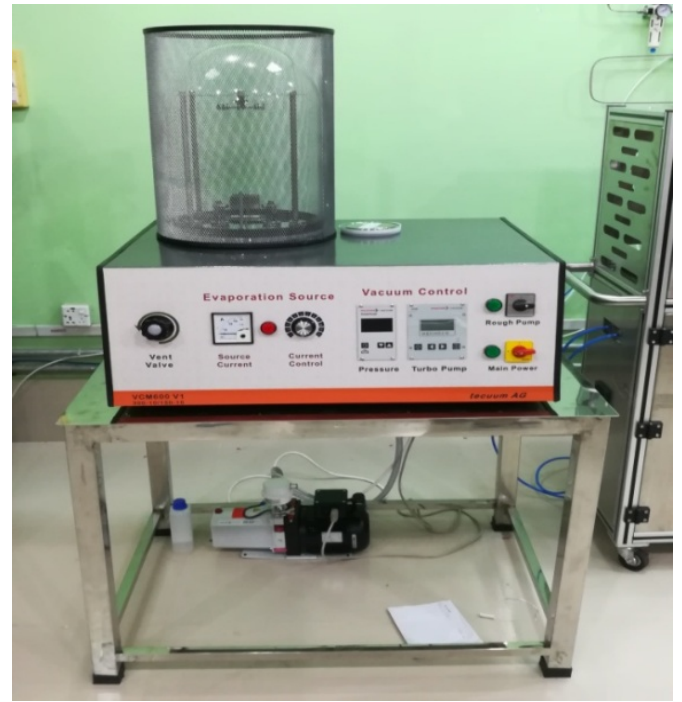
Fig. 2 Full set up of VCM 600 V1 Vacuum Evaporator
