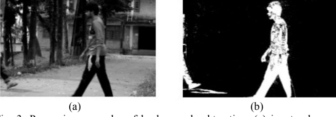
Fig. 3. Processing examples of background subtraction: (a) input enhanced frame, and (b) background subtracted frame.
