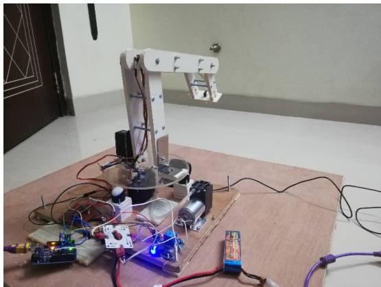
Fig.07: Implementation of the robotic arm
