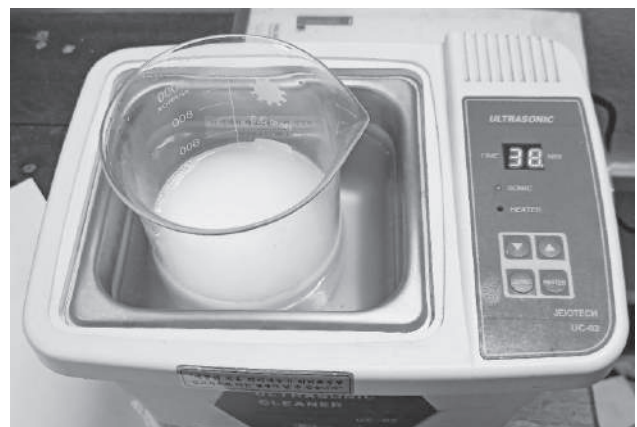
Fig. 7. Ultrasonic Bath to disperse the nanoparticle properly
