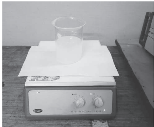
Fig. 6. Magnetic stirrer to mix the nanoparticle to base fluid
