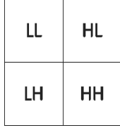
Fig. 1 Single level DWT decomposition of an image.
