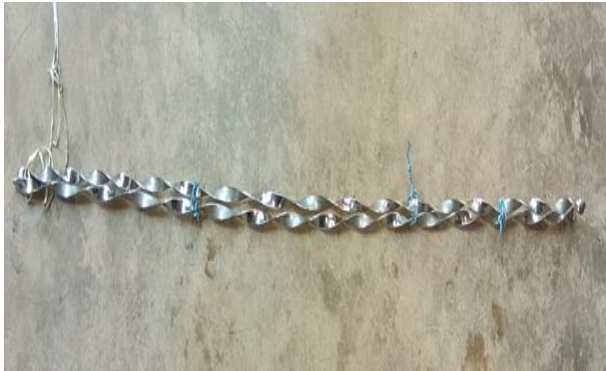
Fig. 1 Photographic view of double counter twisted tape
