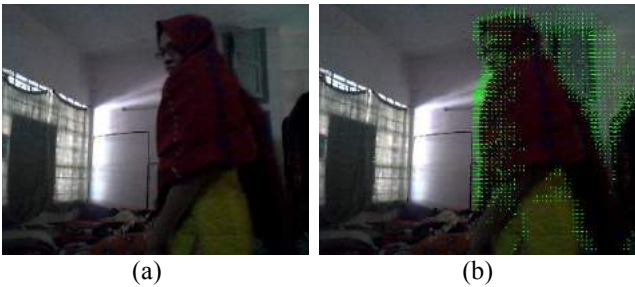
Figure 7: Motion estimation of record1.avi (frame-34) (indoor-day): (a) original; (b) motion vector
