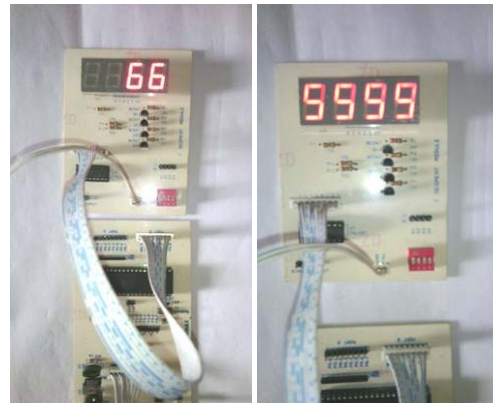
Fig. 14 7 Segment Module Testing Result Output.
