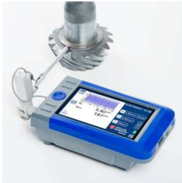
Figure 3.13: Taylor Hobson Ametex Surface roughness tester
