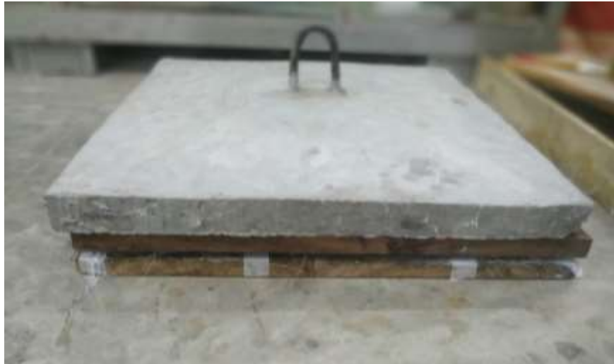
Figure 3.10: Weight for compressing the specimen
