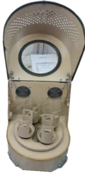
Figure 3.5: Ball milling machine
