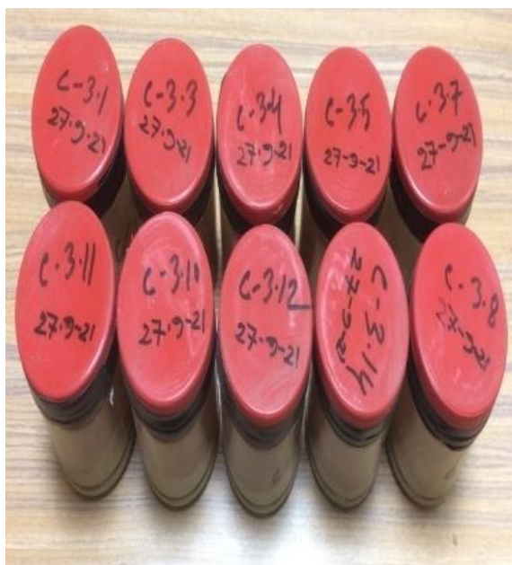
Fig. 3.5: Sample preparation for natural radioactivity measurements.
