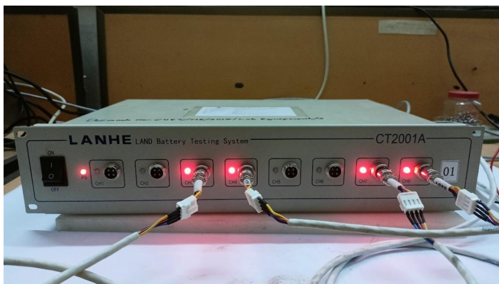
Figure 3.3 LAND battery testing device
