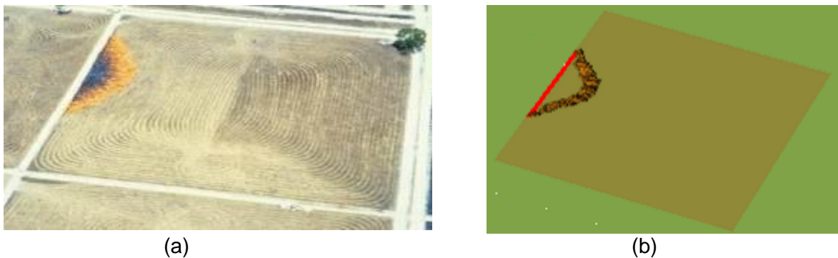
Figure 12: (a) Burning of Australian grassland and (b) CFD-based simulation
