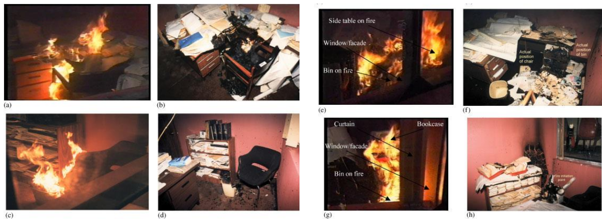
Figure 5. Size of the fire at time of sprinkler activation and resulting damage during Capita Façade tests
