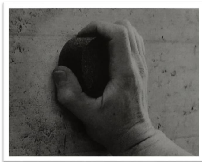
Figure 3.6: Preparing test surface (RHT “Proceq” manufacturer manual; Fewtrell, 1993)
