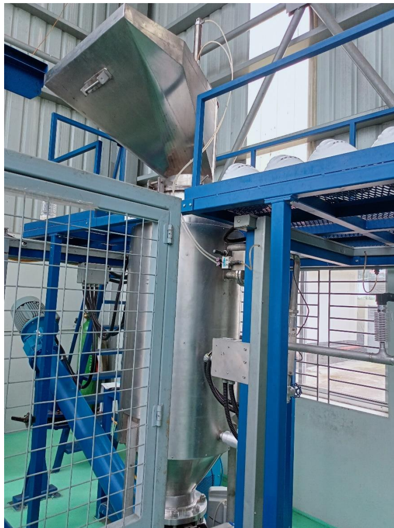
Fig. 3.9: Fixed bed downdraft gasifier.
