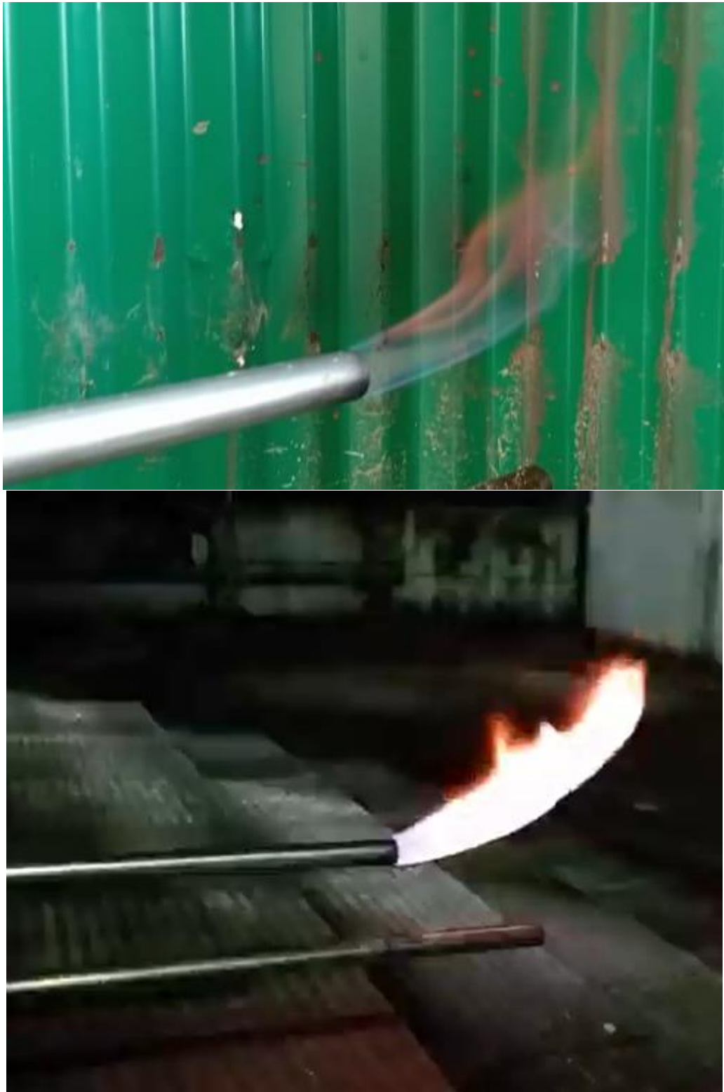
Fig.3.15: Flammability test of the produced syngas.
