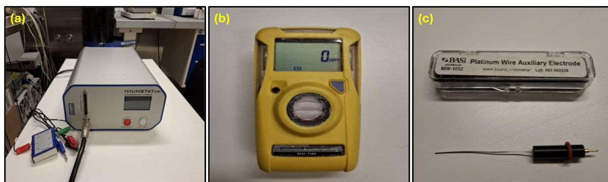
Figure 8. Used instruments in the experiment (a) electrochemical workstation (b) portable single gas detector (c) platinum wire as counter electrode
