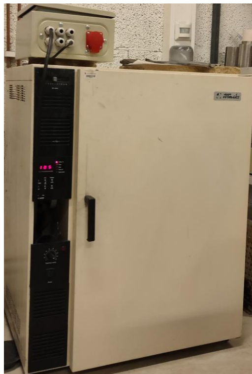
Figure 3.5: Termaks TS4057 laboratory oven
