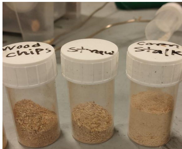
Figure 3.4: Raw samples after grinding in Polymix® System PX-MFC 90 D hammer mill. (Left to right, woodchips, wheat straw and corn stalk, respectively)
