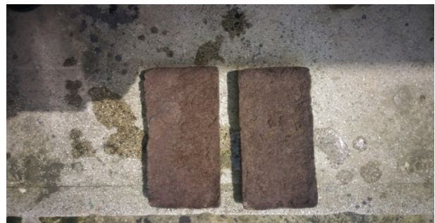
Fig 3: Bangladesh standard sized plastic sand bricks
