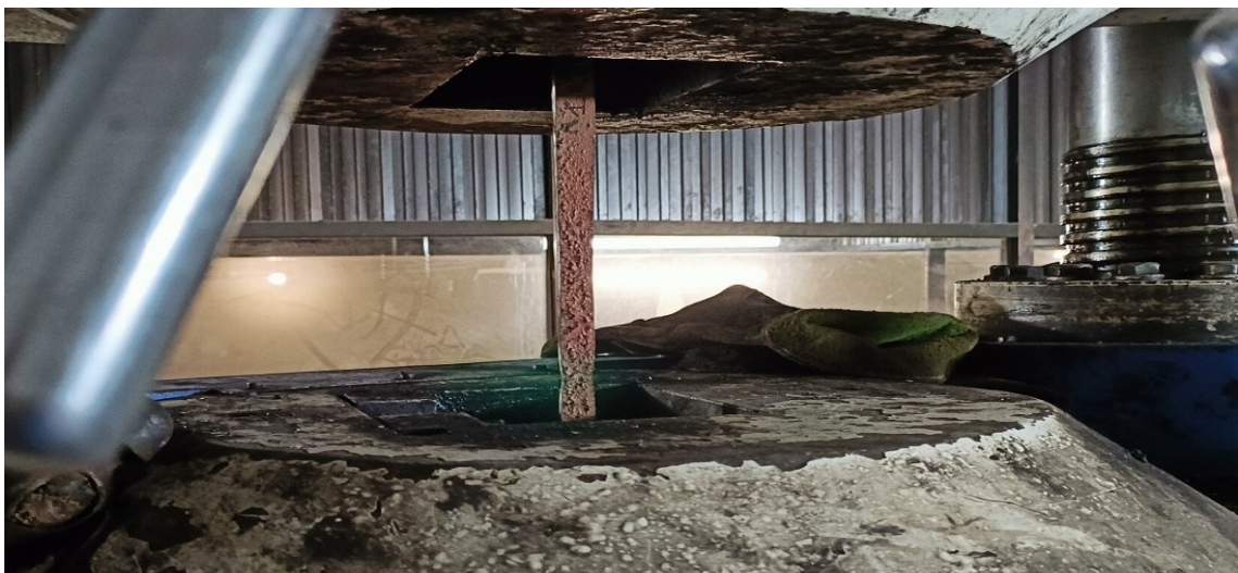
Fig. 3.11. Coupon Test of Metal Beam
