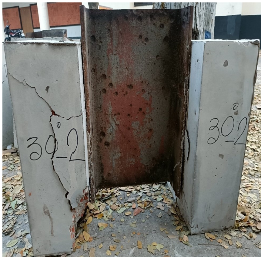
Fig. 4.11. Failure Pattern of HSS_30(2) Specimen
