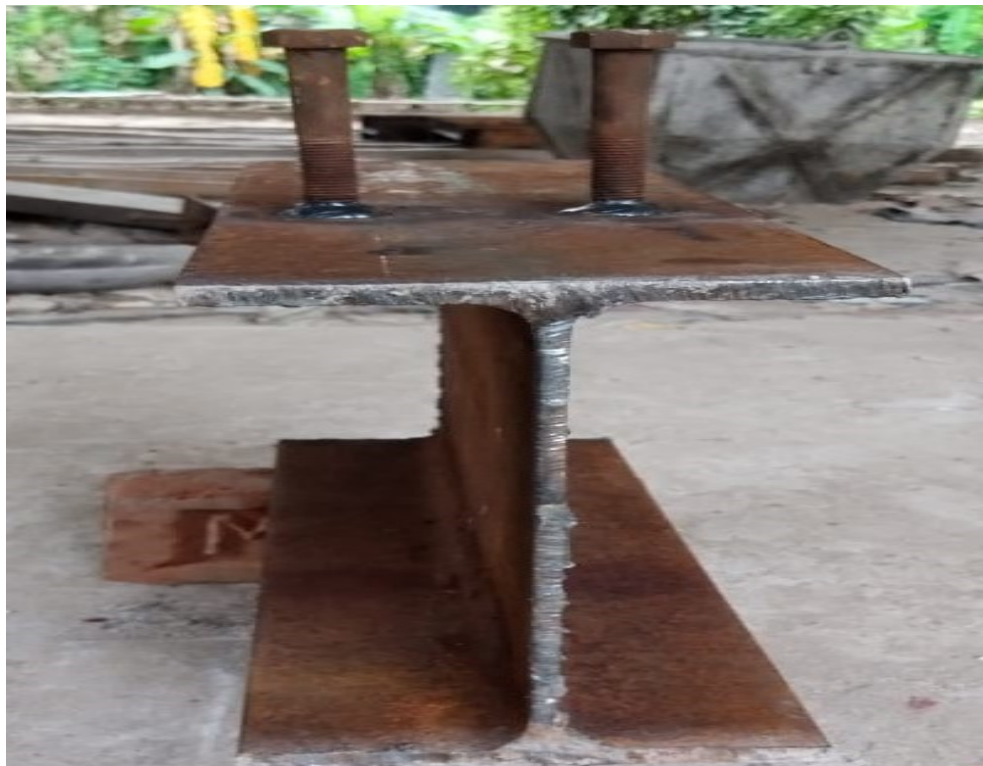
Fig. 3.2. Installed headed shear connector [51]
