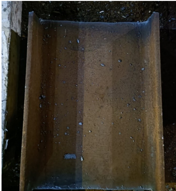
(b) 450mm Length I Shaped Steel Girder (a) 110mm Length headed Shear Stud
