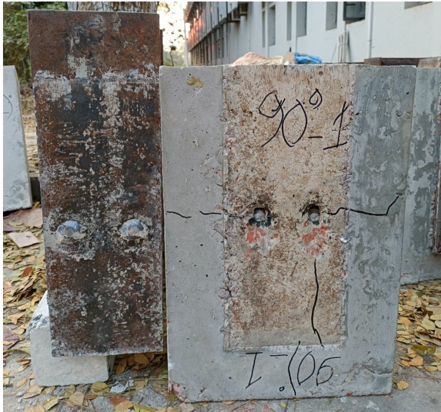
Fig. 4.2. Failure Pattern of HSS_90(1) Specimen
