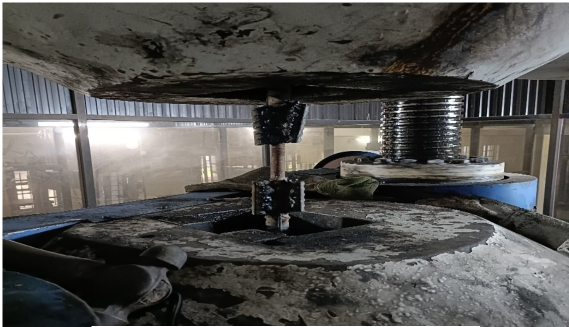
Fig. 3.12. Tensile Potency Test of Stud Connector
