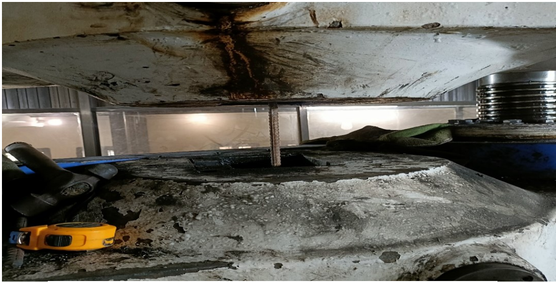
Fig. 3.13. Tensile Potency Test of 12mm dia Rod
