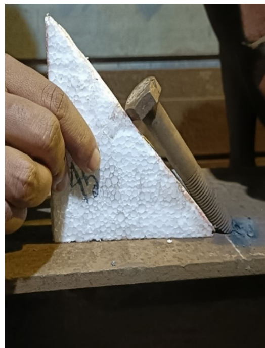
(b) Using formwork during welding Rod
