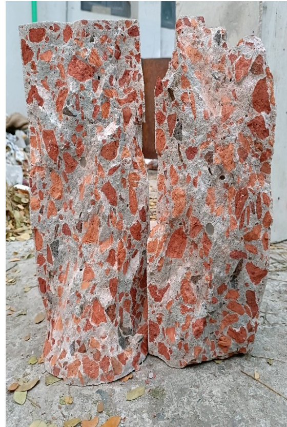
Fig. 3.10. Failure Pattern of Concrete Cylinder
