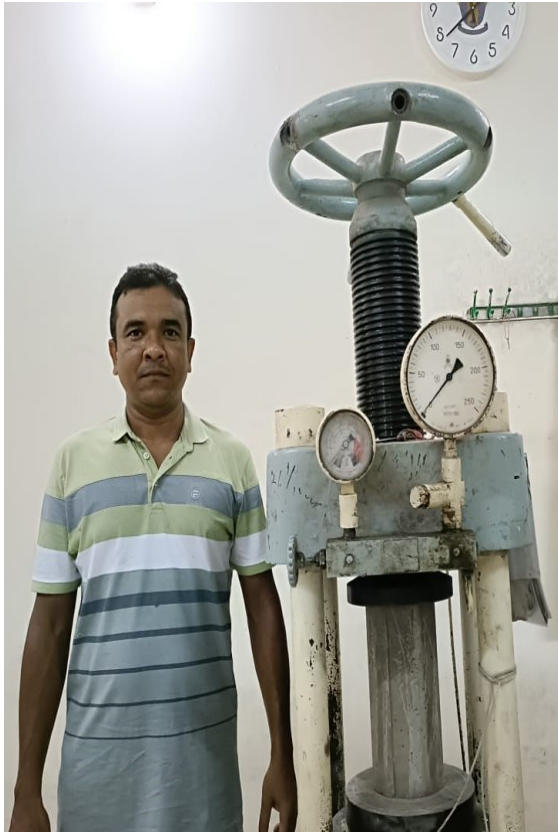
Fig. 3.9. Concrete Cylinder Set up
