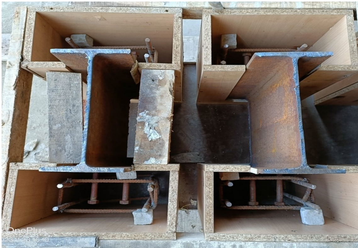
Fig. 3.22. Push Out Specimen's Formwork Ready for Oiling Before
