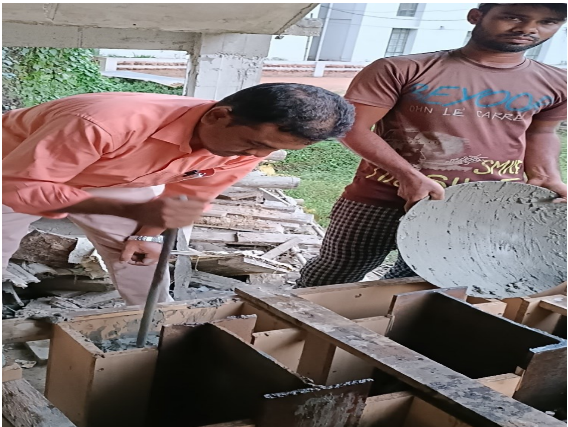
Fig. 3.26. Tamping During Pouring of Concrete to the Specimen
