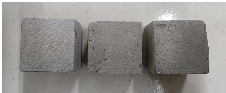
Fig. 3.5. 2"x2"x2" Cube for Compressive Strength Test of Cement
