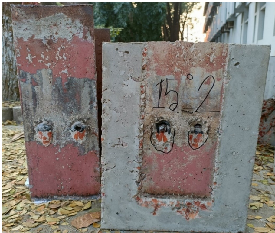
Fig. 4.7. Failure Pattern of HSS_15(2) Specimen
