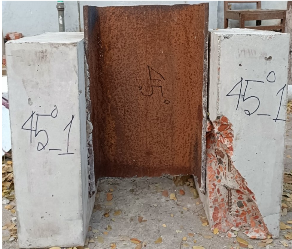
Fig. 4.14. Failure Pattern of HSS_45(1) Specimen
