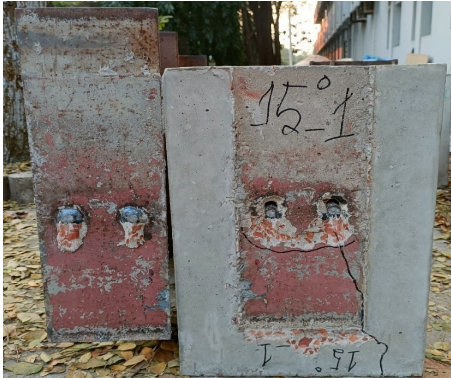
Fig. 4.6. Failure Pattern of HSS_15(1) Specimen
