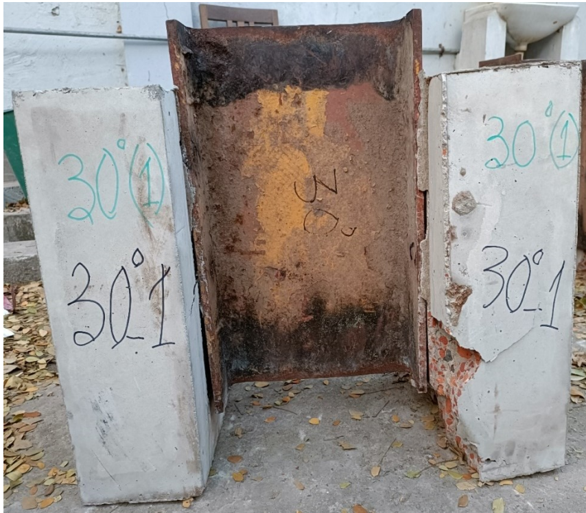
Fig. 4.10. Failure Pattern of HSS_30(1) Specimen
