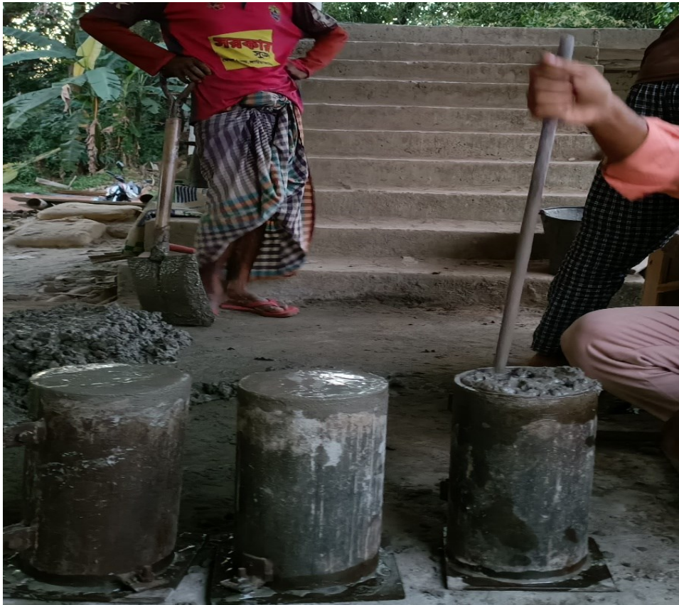
Fig. 3.27. Randomly Collecting Cylinder Test Sample During
