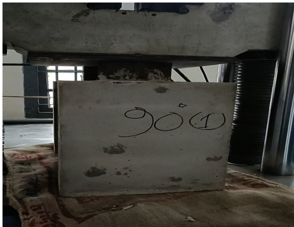
Fig. 3.32. Typical Sample of Specimen Testing on UTM
