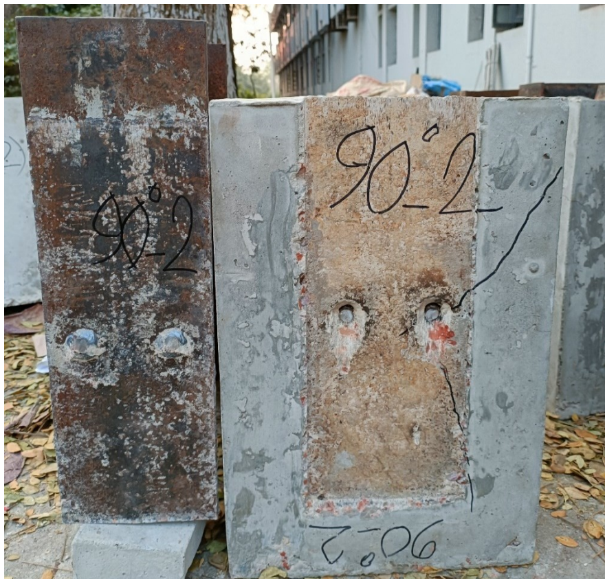
Fig. 4.3. Failure Pattern of HSS_90(2) Specimen
