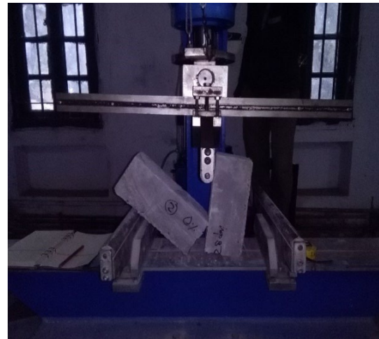
(b) Concrete Beam Flexural test (after loading)
