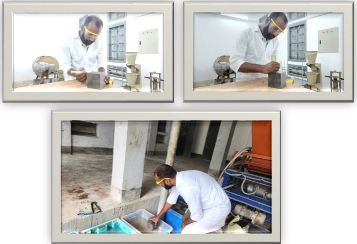
Figure 3.3: Curing of the specimen
