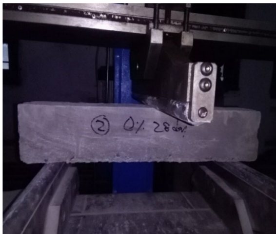
(a) Concrete Beam Flexural test (before loading)
