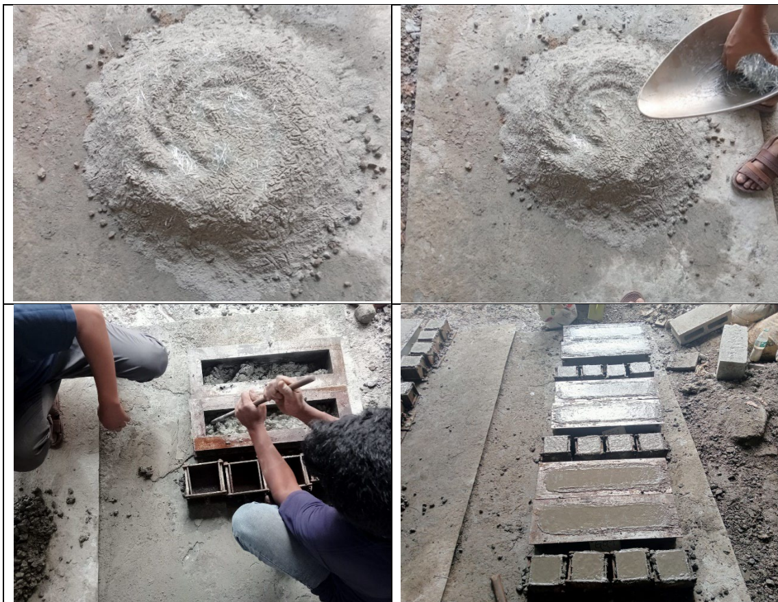
Figure 3.2: Casting of cube & prism specimen for different curing ages
