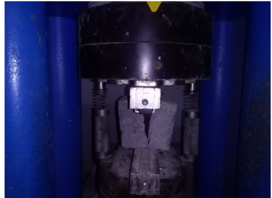
Figure 3.7: Test apparatus for determining concrete split tensile strength
