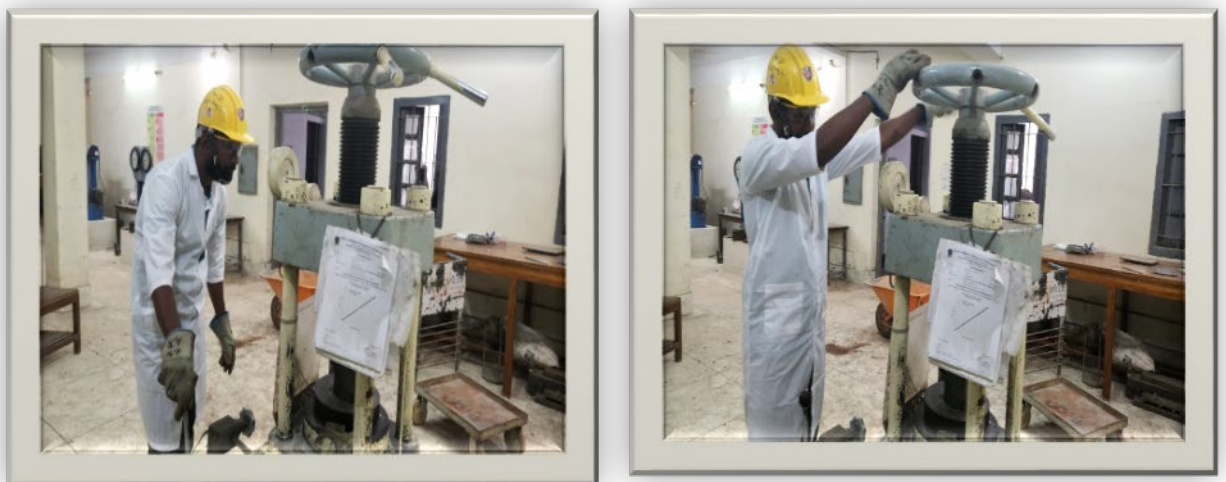
Figure 3.5: Test setup for determining concrete cube compressive strength.
