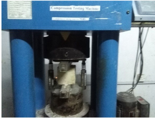
Figure 3.7: Test apparatus for determining concrete split tensile strength
