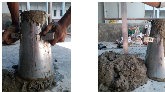
Figure 3.18: Workability of concrete (Slump test)
