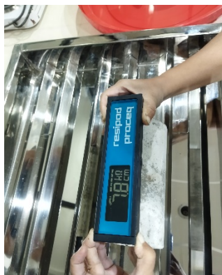
Figure 3.23: Surface electrical resistivity test setup
