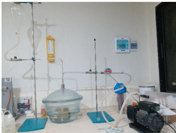
a) Vacuum saturation setup
