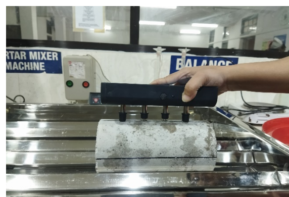
Figure 3.23: Surface electrical resistivity test setup
