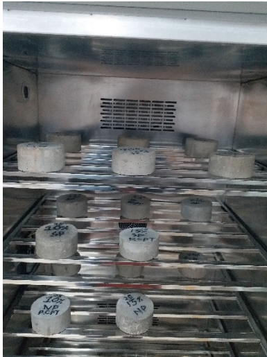
a) Samples in humidity chamber
