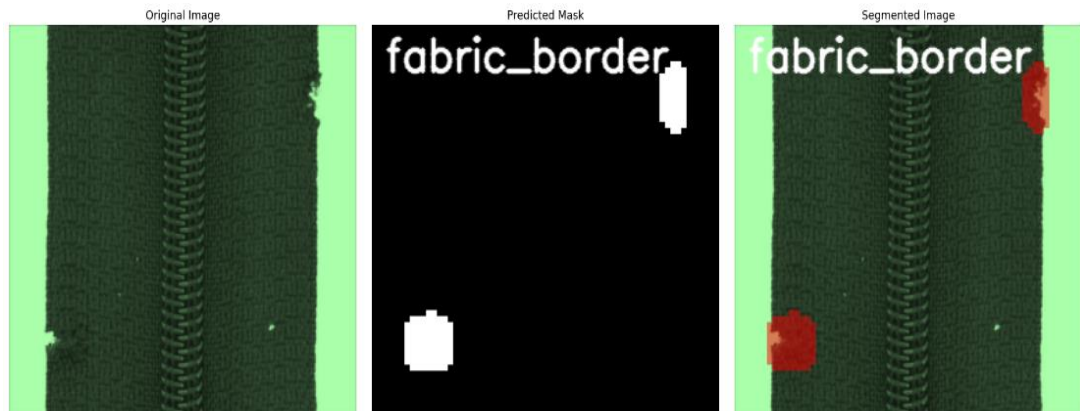
Figure 4.116: Fabric border defect of zipper
