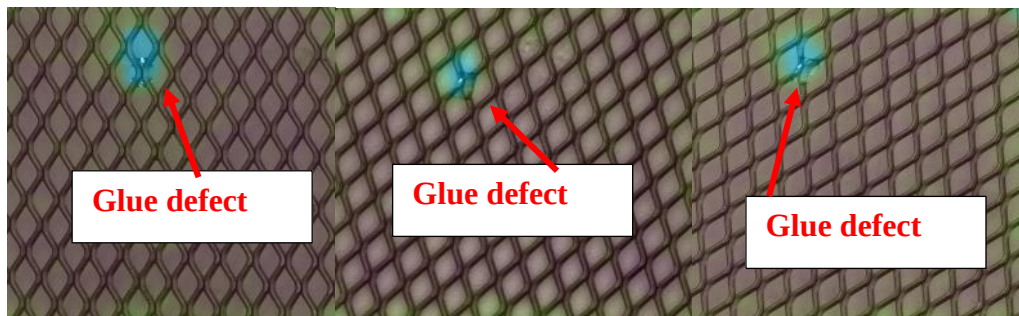
Figure 4. 7: Glue defect of Grid
