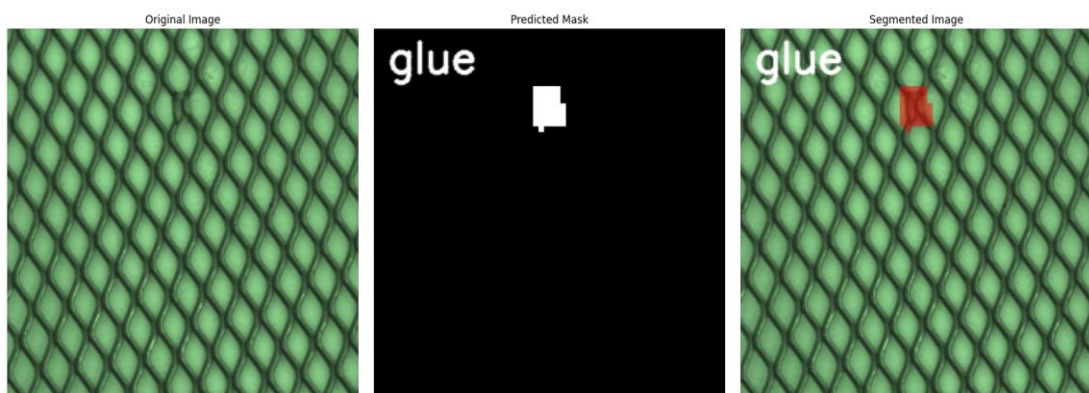
Figure 4.91: Glue defect of grid
