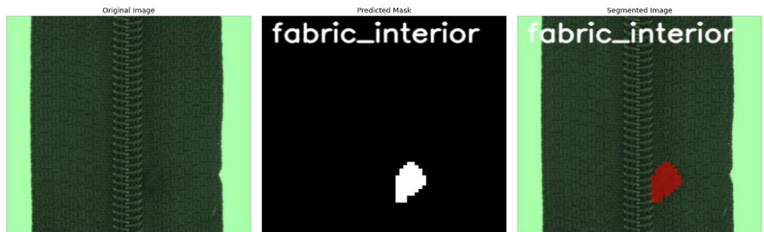
Figure 4.117: Fabric interior defect of zipper
