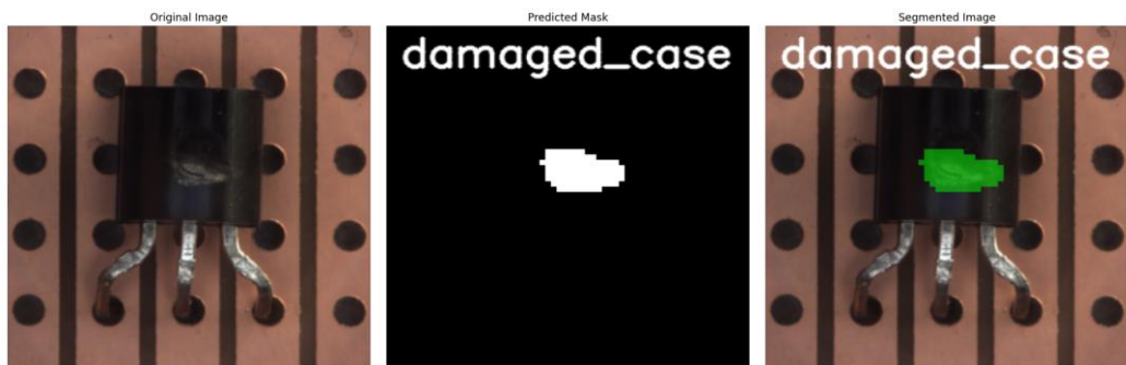
Figure 4.111: Damaged case defect of transistor
