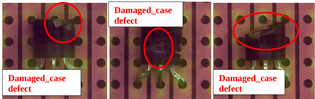
Figure 4. 23: Damaged_case defect of transistor
