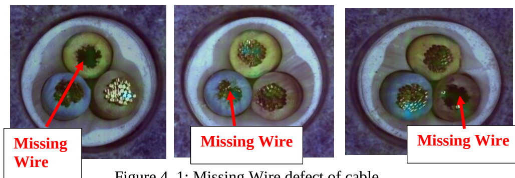
Figure 4. 1: Missing Wire defect of cable
