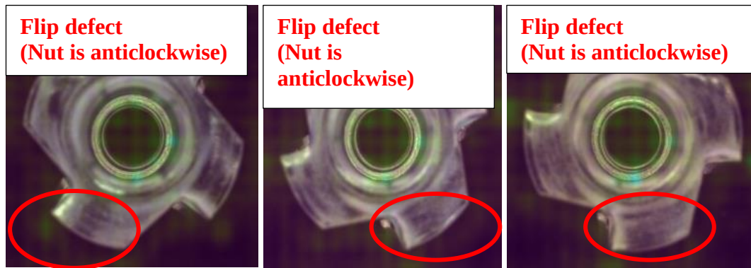
Figure 4. 14: Flip defect of metal nut
