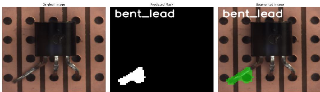
Figure 4.109: Bent lead defect of transistor
