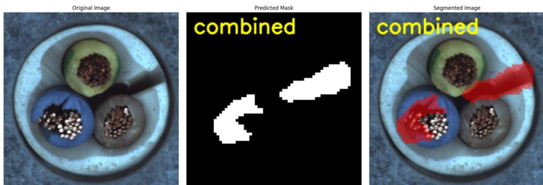
Figure 4. 36: Combined defect of cable
