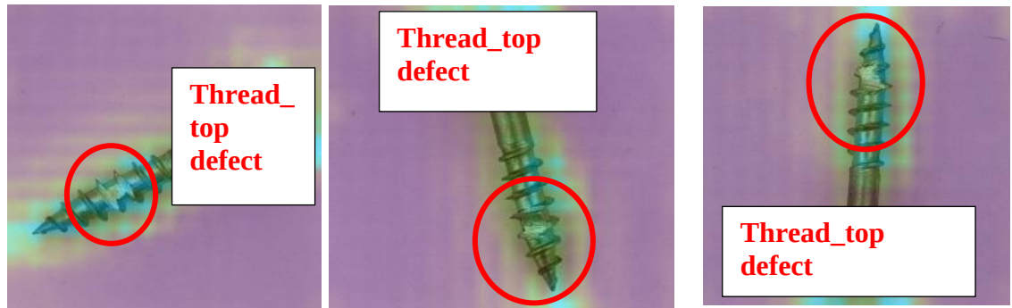
Figure 4. 19: Thread top defect of screw
