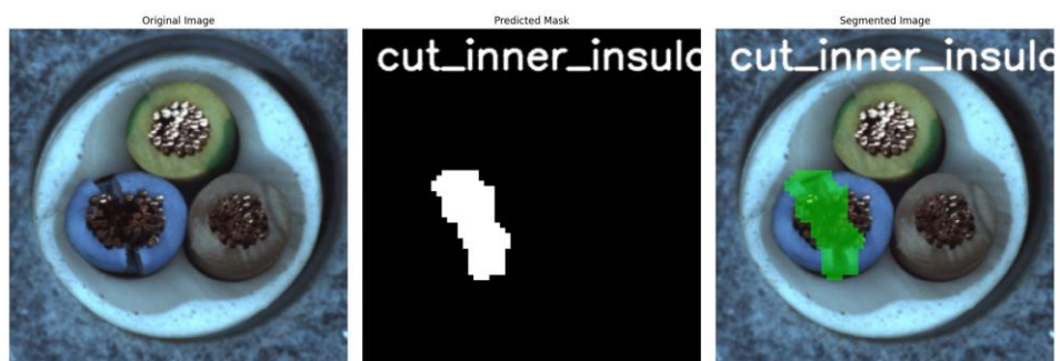
Figure 4.81: Cut inner insulation defect of Cable
