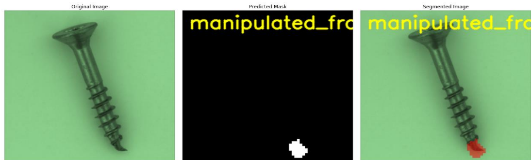
Figure 4. 57: Manipulated front defect of screw
