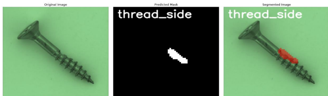
Figure 4.105: Thread side defect of screw
