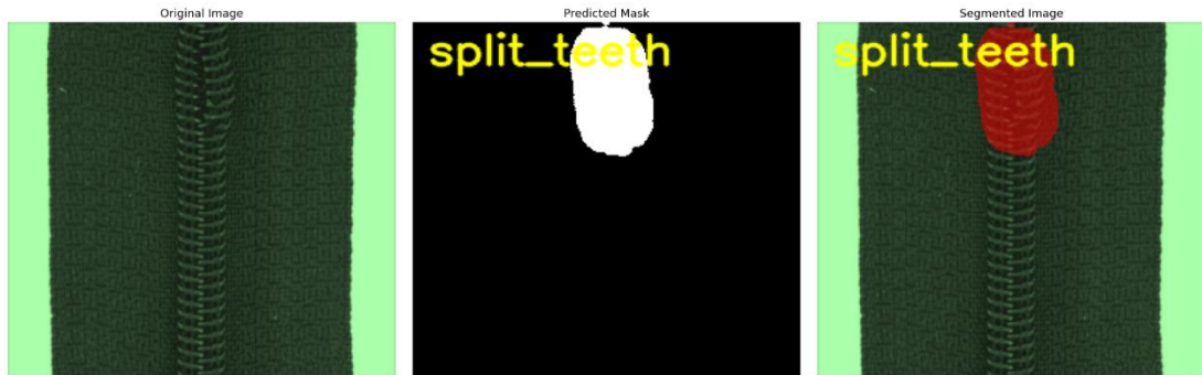
Figure 4. 75: Split teeth defect of zipper
