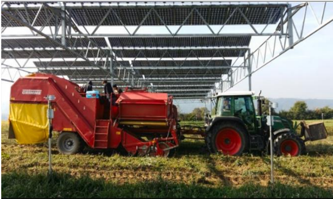
Fig. 2.6: Potato harvesting under APV panels in 2017 (Source: farm community Heggelbach) [93].
